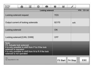
Figure 4-13 Sample Active Test Screen
