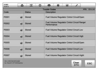
Figure 4-17 Sample DTC & FFD Screen
