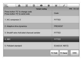
Figure 4-14 Sample Variant Coding Screen
