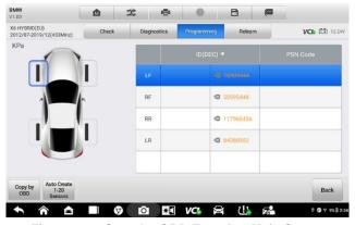
Figure 5-25 Copy by OBD Function Main Screen
