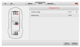
Figure 7-10 Starter Test Result Screen
