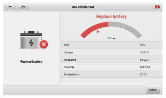
Figure 7-14 Sample Out-vehicle Test Result Screen
