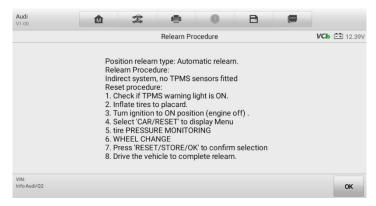
Figure 5-13 Relearn Procedure for Indirect TPMS
