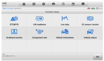
Figure 4-18 OBDII Diagnostic Menu
