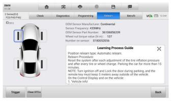
Figure 5-27 Relearn Function Main Screen
