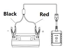
Figure 7-2 Connecting to a Battery
