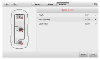
Figure 7-12 Generator Test Result Screen
