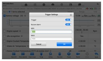
Figure 4-14 Trigger Setting Dialog Box
