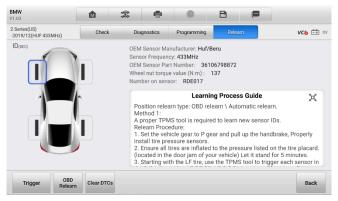
Figure 5-26 Relearn Function Main Screen
