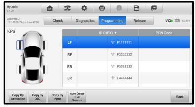
Figure 6-26 Copy by Activation Confirmation Screen
