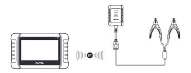
Figure 13-3 Battery Tester Connection Example 1
