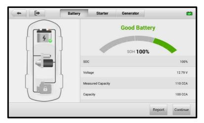
Figure 13-7 Battery Test Results Screen
