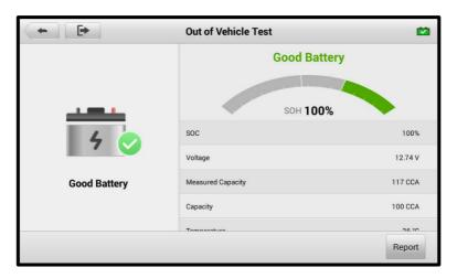
Figure 13-11 Out-vehicle Test Results Screen
