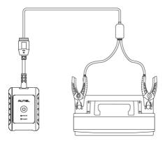
Figure 13-4 Battery Tester Connection Example 2
