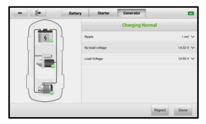
Figure 13-9 Generator Test Results Screen
