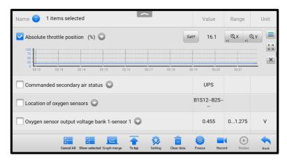
Figure 4-15 Waveform Graph Mode Screen
