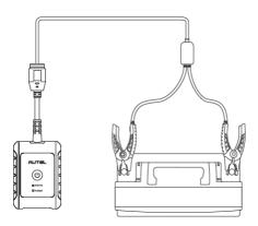
Figure 13-4 Battery Tester Connection Example 2
