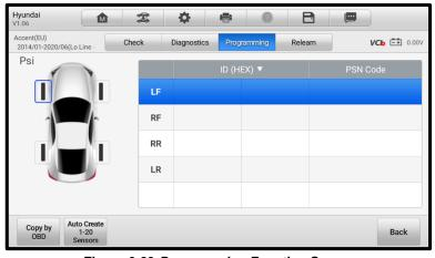
Figure 6-23 Programming Function Screen
