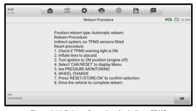
Figure 6-12 Relearn Procedure for Indirect TPMS
