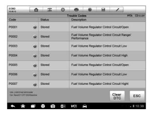
Figure 4-18 Sample DTC & FFD Screen
