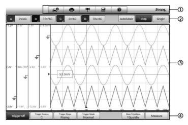
Figure 15-4 Sample MaxiScope Application Screen Layout
