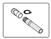
Screw the thread part of the accessory over the imager head to fix the accessory.
