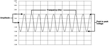
Figure 15-1 Sample Sinusoidal Waveform
