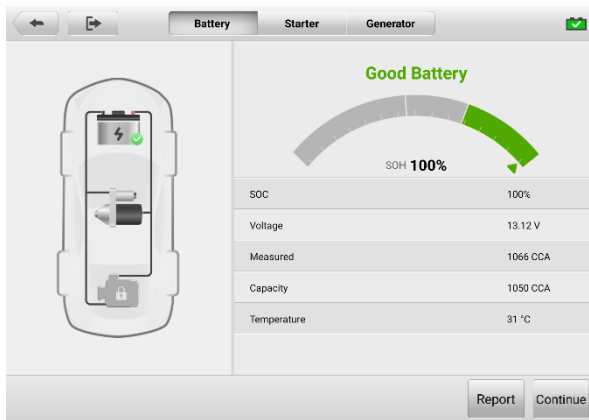
Figure 6-5 Battery Test Results Screen
