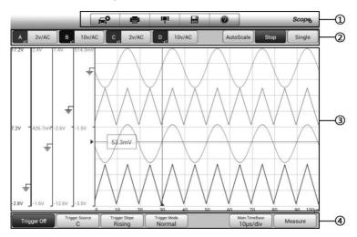
Figure 15-4 Sample MaxiScope Application Screen Layout
