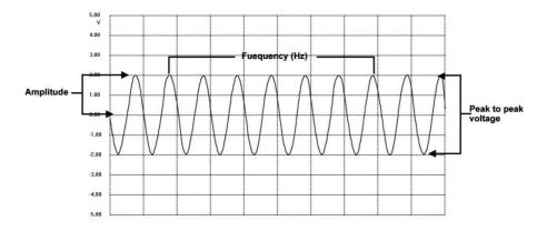
Figure 15-1 Sample Sinusoidal Waveform
