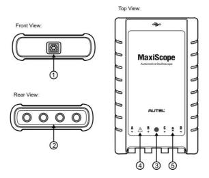
Figure 15-3 Front, Rear, and Top View
