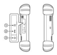
Figure 2-3 MaxiSys Tablet Left Side
