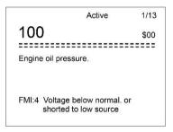
Figure 4-5 Sample DTC Screen
