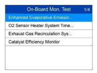
Figure 3-32 Sample On-board Mon. Test Screen 1
