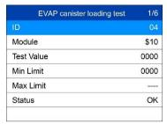
Figure 3-34 Sample On-board Mon. Test Screen 3
