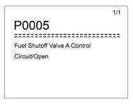
Figure 3-6 Sample DTC Screen
