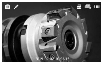
Figure 3-7 USB icon displays when Transfer Files selected
