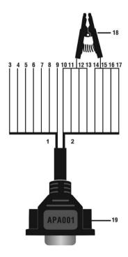
Figure 2-5 EEPROM Clamp Integrated MC9S12 Cable
