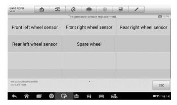
Figure 7-31 Sample Tire Pressure Sensor Replacement Screen
