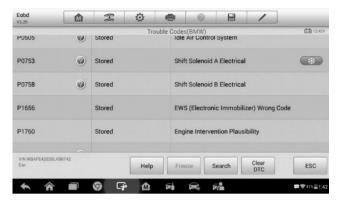
Figure 6-7 Sample DTC & FFD Screen
