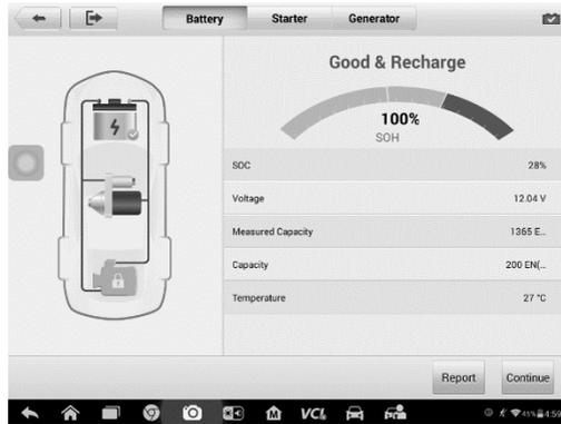
**Figure 17-6 Sample Battery Test Results Screen**
