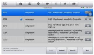
Figure 4-16 Sample DTC & FFD Screen
