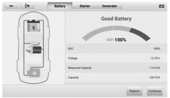
Figure 6-7 Sample Battery Test Results Screen
