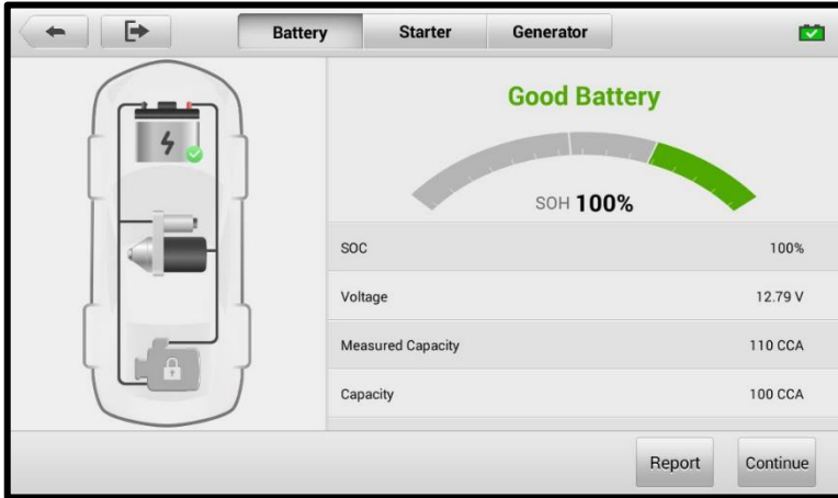
Figure 10-7 Battery Test Results Screen
