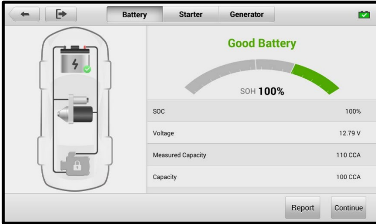
Figure 12-7 Battery Test Results Screen
