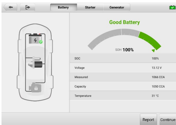
Figure 10-6 Battery Test Results Screen
