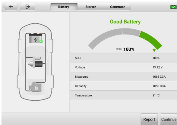
Figure 10-6 Battery Test Results Screen
