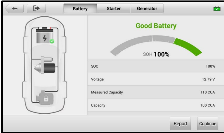
Figure 10-7 Battery Test Results Screen
