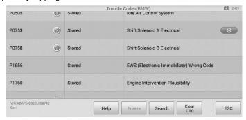
Figure 4-19 Sample DTC & FFD Screen
