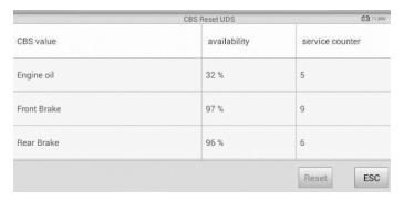
Figure 6-4 Sample Oil Reset Service Screen 3
