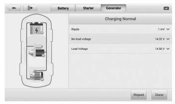
Figure 7-10 Sample Generator Test Results Screen
