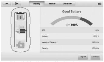
Figure 7-7 Sample Battery Test Results Screen
