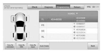
Figure 5-20 Sample Copy by Activation Complete Screen
