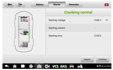
Figure 4-6 Sample Starter Test Result Screen Table 4-3 Starter Test Results
