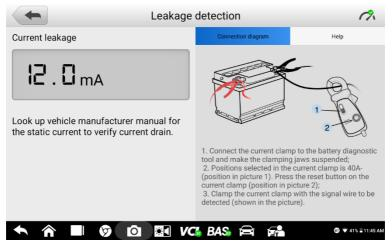
Figure 11-2 Sample Leakage Detection (Current Model) Screen
