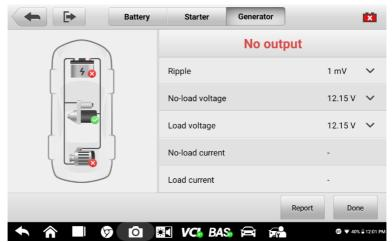
Figure 4-7 Sample Generator Test Result Screen
