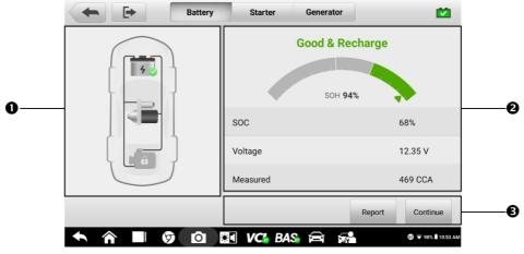
Figure 4-5 Sample Battery Test Result Screen
