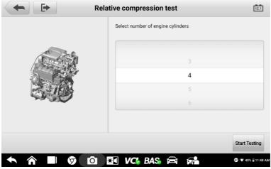
Figure 11-4 Sample Relative Compression Test Screen
