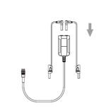
Plug the red test lead into the red color coded input of the multimeter, and the black test lead into the black input.
