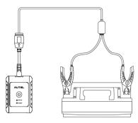
Figure 10-3 Connecting to a Battery
