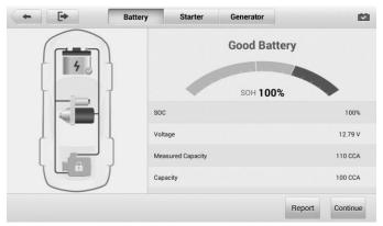
Figure 10-7 Sample Battery Test Results Screen
