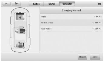
Figure 10-10 Sample Generator Test Results Screen
