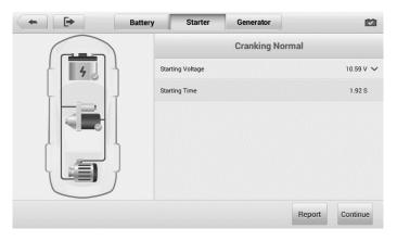
Figure 10-9 Sample Starter Test Results Screen
