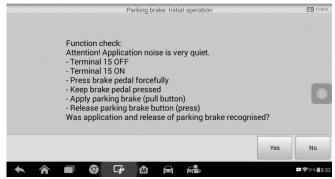
Figure 5-7 Sample Parking brake: Initial operation Screen 1
