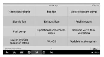
Figure 4-16 Sample Active Test Screen
